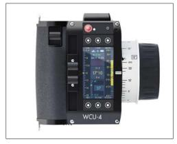
One of the most groundbreaking new features of the WCU-4 is the option to use Vibration-Markers, which provide haptic feedback for electronic markers and limits. Essentially, focus pullers can set soft rather than hard stops, and the unit will vibrate to warn them when they are at their pre-set limits or stops. This allows them to keep their eyes on the performers at all times, leading to greater accuracy of focus.
